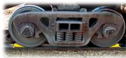
With Wheel Wedge the wheel is blocked with no more debris left on the track when the car is pushed over the wedge.
